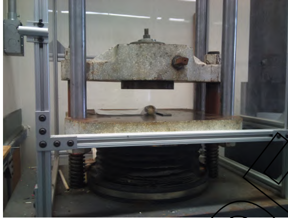
Figure 2: Compression testing machine with sugar cane sample loaded
