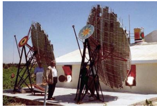
Figure V.i.4 Scheffeler solar community collector [19]
