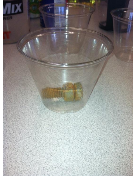
Figure 2: Acetone corrosion removal test
