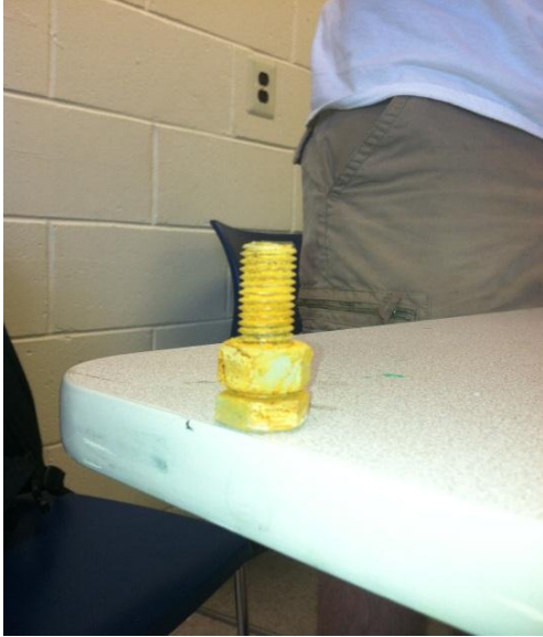
Figure 1: Rusted 1/4 inch bolt
