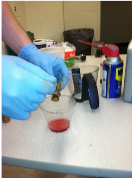
Figure 3: Coating of 100% ATF onto corroded bolt.
