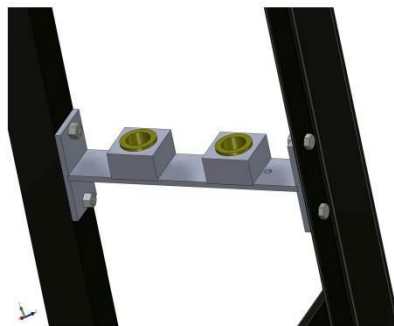
Figure 2 – Roller Bushings Installed
