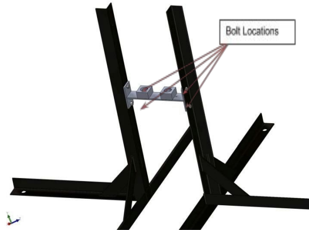
Figure 1 – Bottom Base Installed
