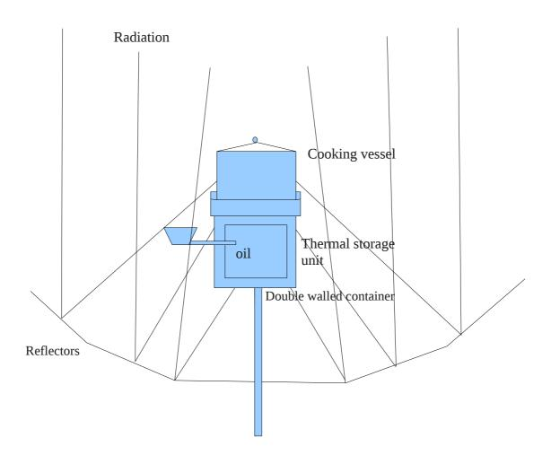
In order to understand the functioning of the cooker at night, the interior of the double walled vessel has to be looked into in a more detailed manner.
