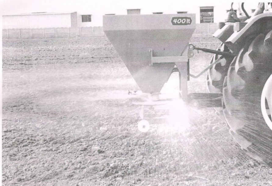
Fig. 5: Fertilizer Broadcaster being used for broadcasting DAP
