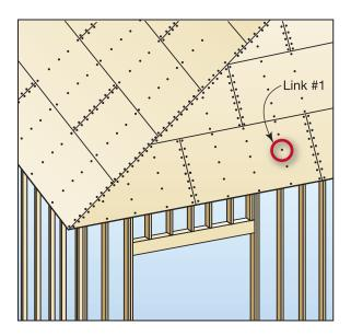
is significantly greater than that provided by a smooth shank nail. Additional strength can be added by using ring shank nails, also called deformed shank nails. The grooves and ridges along the shank act as wedges, giving the nail more withdrawal strength than a typical smooth shank nail.
