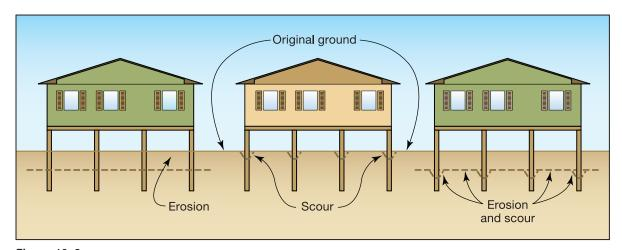
Figure 10-6. Scour and erosion effects on piling embedment
