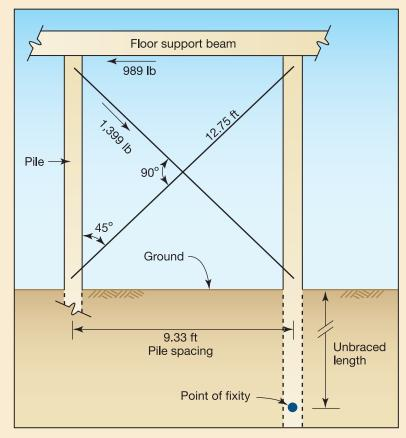
Illustration A. Force diagram for diagonal bracing
