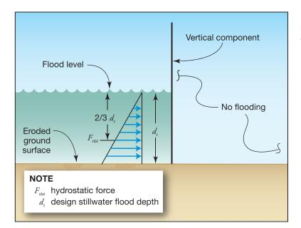
Figure 8-7. Lateral flood force on a vertical component
