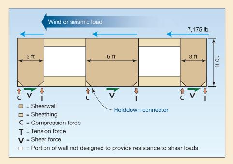
Illustration A. Loads on south shear wall
