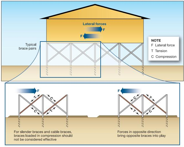
Figure 10-11. Diagonal bracing schematic
