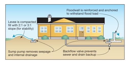
Figure 15-13. Home protected by a floodwall and a levee
