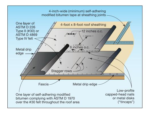
is to avoid leakage into the residence if the felt blows off or is torn by wind-borne debris. (Taping the joints is not included in the first variation, shown in Figure 11-26, because with the self-adhering modified bitumen sheet applied directly to the sheathing, sheet blow-off is unlikely, as is water leakage caused by tearing of the sheet by debris.)
