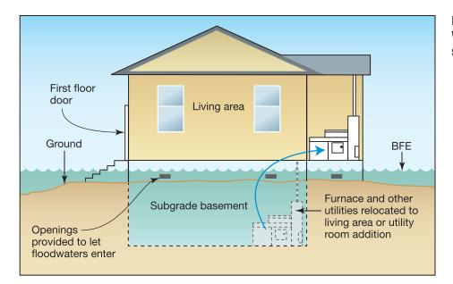
Figure 15-12. Wet floodproofed structure
