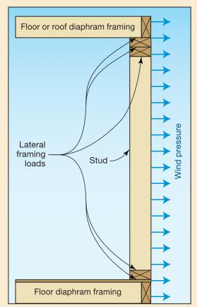
Illustration A. Lateral connector loads for wall-to-roof and wall-to-floor connections
