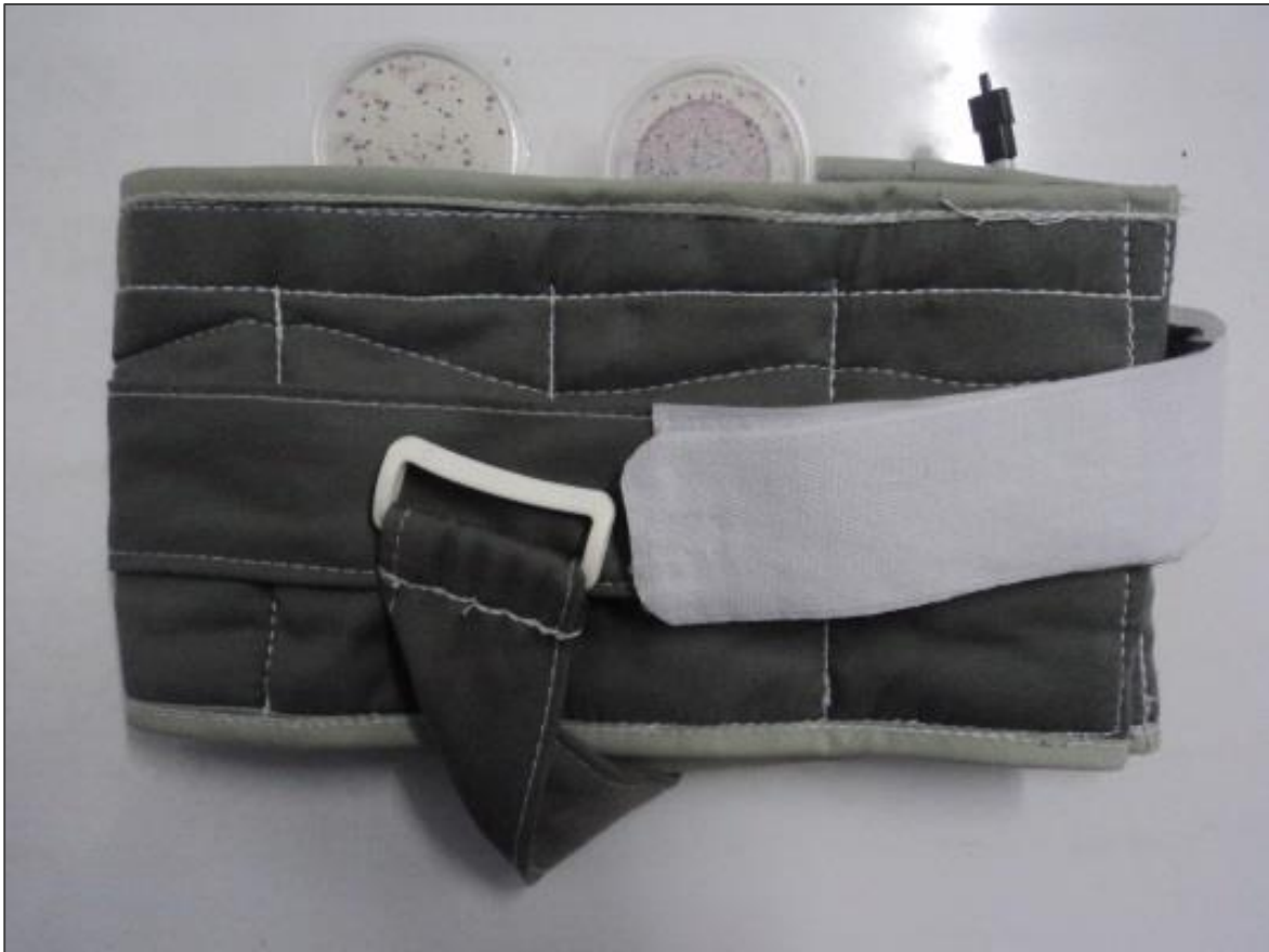
Portable Body Belt incubator developed at ENPHO ; shown along are two media plates with coliform growth and a thermometer on the right
