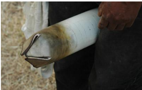
Figure 15 – Bottom of filter heated and bent
