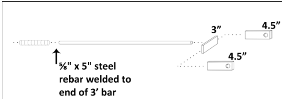
Figure 20 - Exploded view of piston rod
