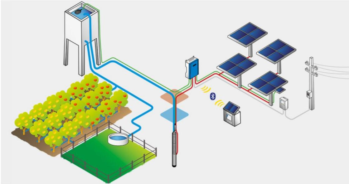
Figure 8: Solar water pumping system designed and manufactured by Lorentz. The model shown is the PS2, comprising a specialized solar pump controller, water pumps and smart sensors to optimize the efficiency of the system.
