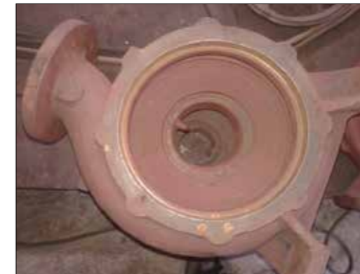
Casing of Pump
