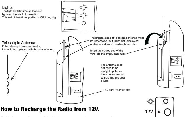
If 12V power is available either from an adaptor or car battery, use the correct plug with 2.1mm centre pin positive (+), and insert it into the correct hole on the side of the radio. Unplug the 12V power when charging is complete. Do not charge for more than 8 hours.
