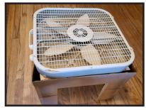
STEP 9: Place your 20-inch box fan on top of the filter face down so that it blows down through the filter
