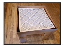
STEP 8: Place your 4x20x20 MERV 13 filter in the frame face down
