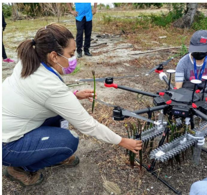
*A WeRobotics drone with a payload box attached*
