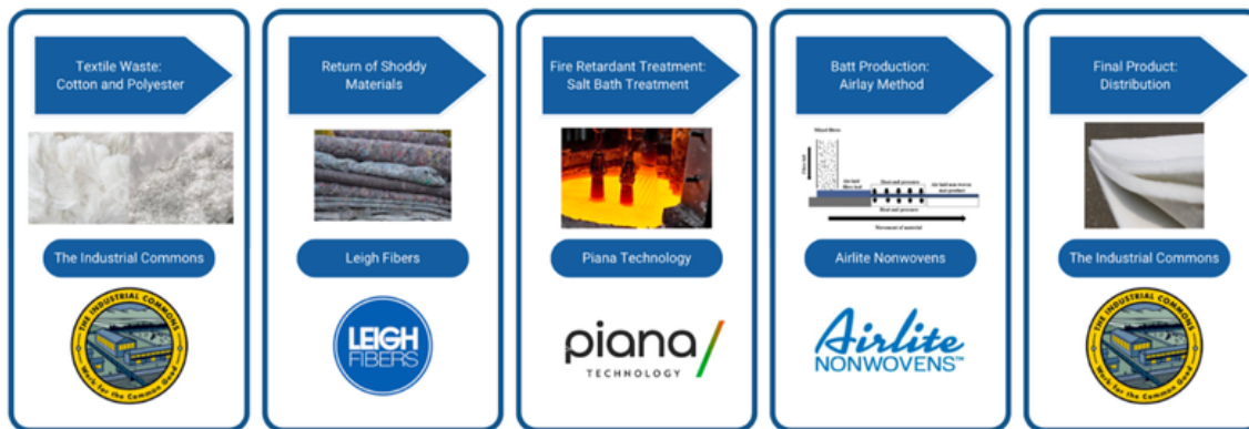
Proposed supply chain for manufacturing of insulation material based on textile waste
