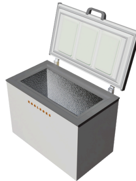
CAD design of Koolboks' 540 litre freezer used for preliminary design phase. Attribution: Oluwatobi Oyeshile
