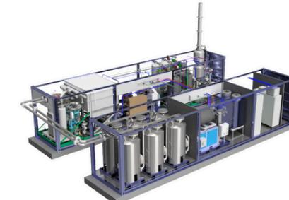
**M2X Containerized Gas Clean-up System with the two 40ft containers placed side by side**
